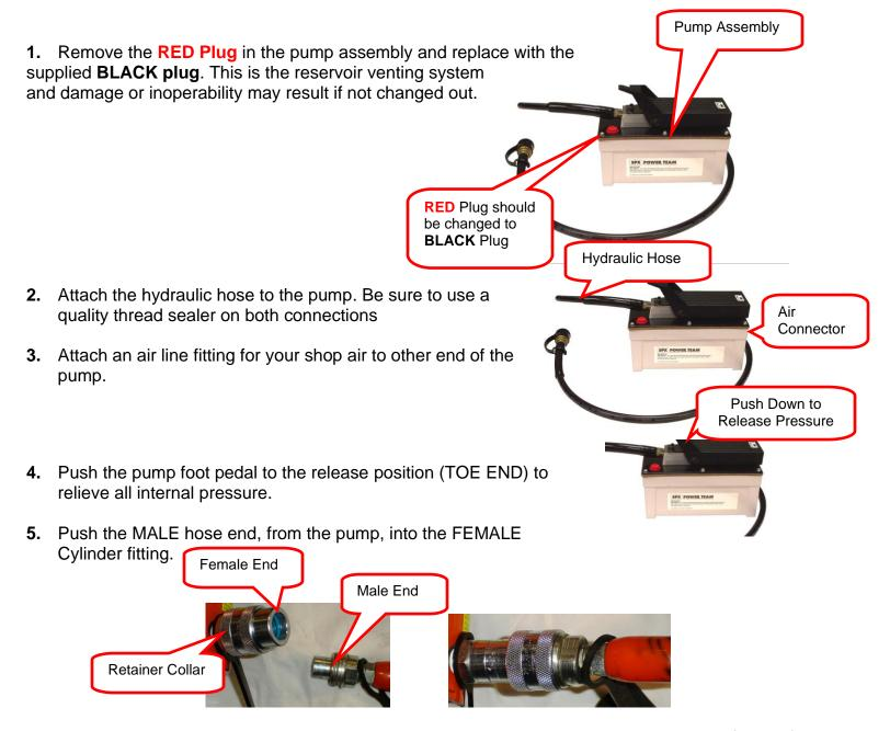
**6.** Thread the retainer collar hand tight. **NOTE:** This procedure will insure that the male & female fittings positively seat against each other, eliminating any possibility of air locking. **CAUTION** Failing to follow this procedure may cause the cylinder to not retract and / or leak.
