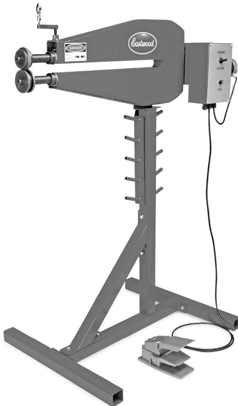
The **Eastwood Motorized Bead Roller** is a professional metal fabrication tool. It is excellent for producing strengthening ribs in replacement floor pans, firewalls, trunk floors, inner fenders, and more. With its full range of bead mandrels, it can also create decorative custom designs in door panels, dashes and much more. Channels and flanges can be formed using offset flange mandrels.
