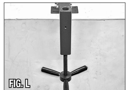
**IMPORTANT NOTE:** The tip of the Pushrod Set-Screw must be seated in the Pushrod Groove sufficiently to prevent the Pushrod from rotating but not too tight, which would prevent free vertical movement.
