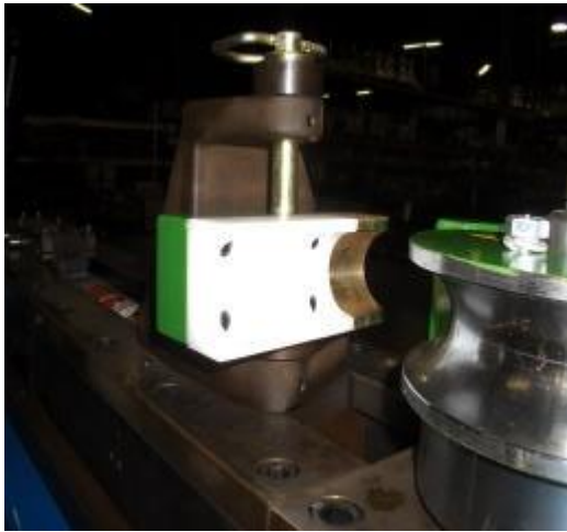
Installing counterdie with 3/4" pin
