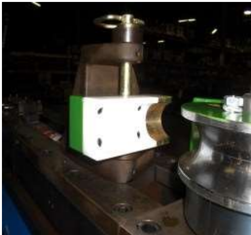
Installing counterdie with 3/4" pin
