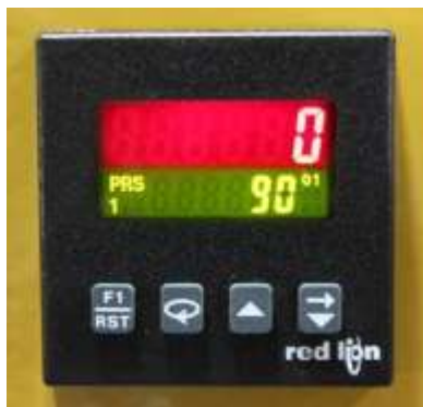
Home position with 90° Preset Stop Point.
