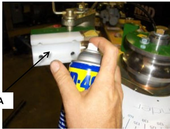
Lubricating counter die bending
