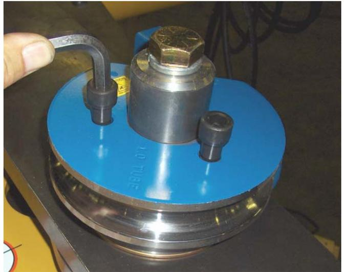
4. To install the counter die, remove the hitch pin (H) and insert the counter die in the opening in the counter die mount until the 3/4" holes line up.
