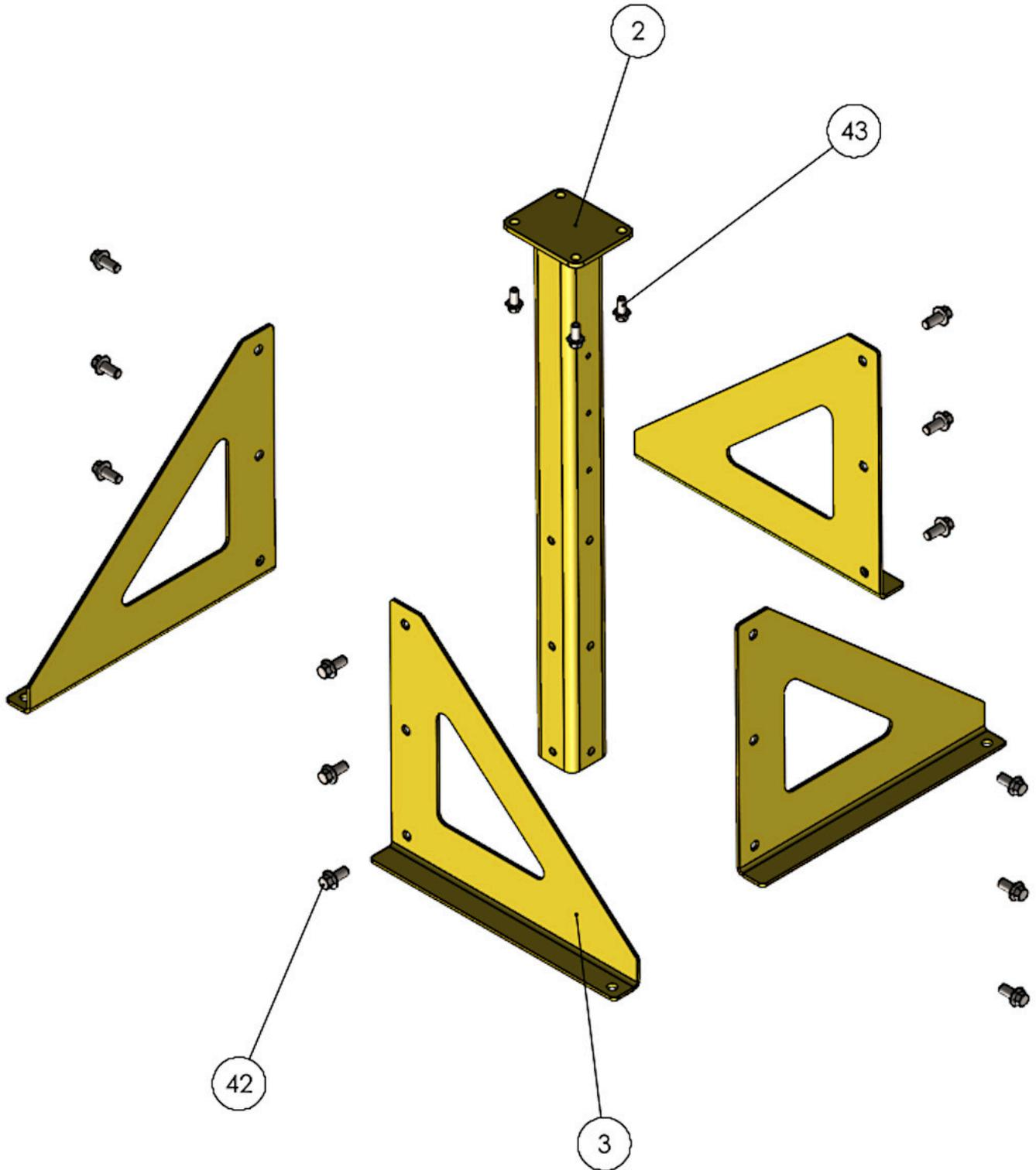
**Main Frame Assembly Parts Diagram**
