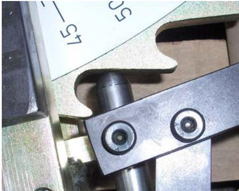
Anti-springback lever engaged
