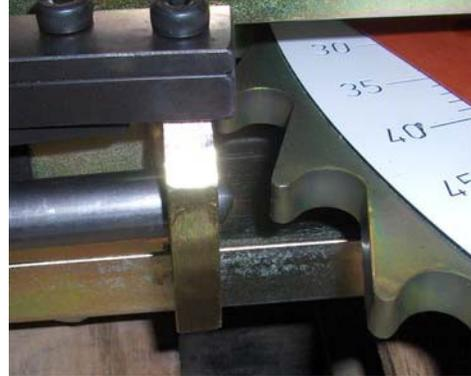
Anti-springback lever disengaged
