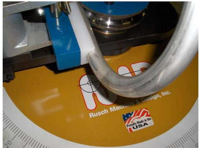
**⚠ IMPORTANT:** Orienting your material in this fashion will cause damage to your tooling and machine!! **DO NOT** pull bent material into the counter die! Make sure you have enough straight material on the draw side of the material to create your bend.
