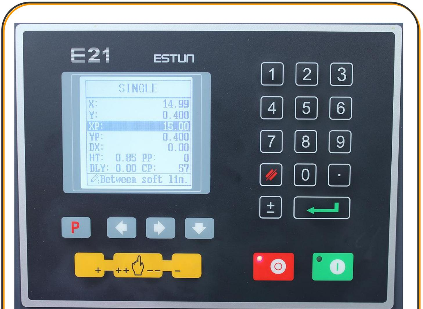
For the first time testing, select “INCH” mode to test the machine actions, and then test “Semi-Auto” mode and the ram stroke adjustment, the back-gauge control etc. Only when the machine actions are confirmed to be completely correctly, operation can be done as per the following procedures:
